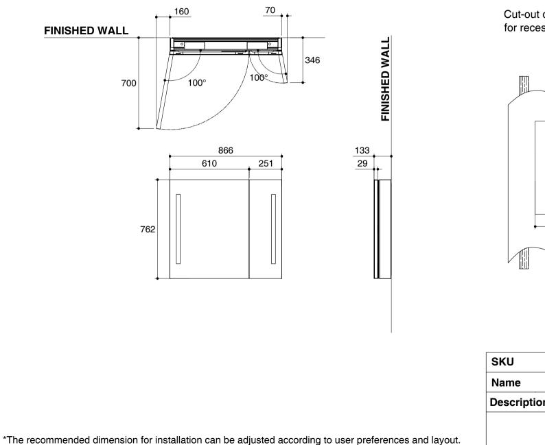
Cut-out dimensions for recess-mount installation
